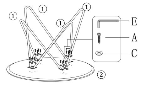
The legs have 2 distinct ends. One 1 end there is only a small hole on the inside and no hole on the outside.
